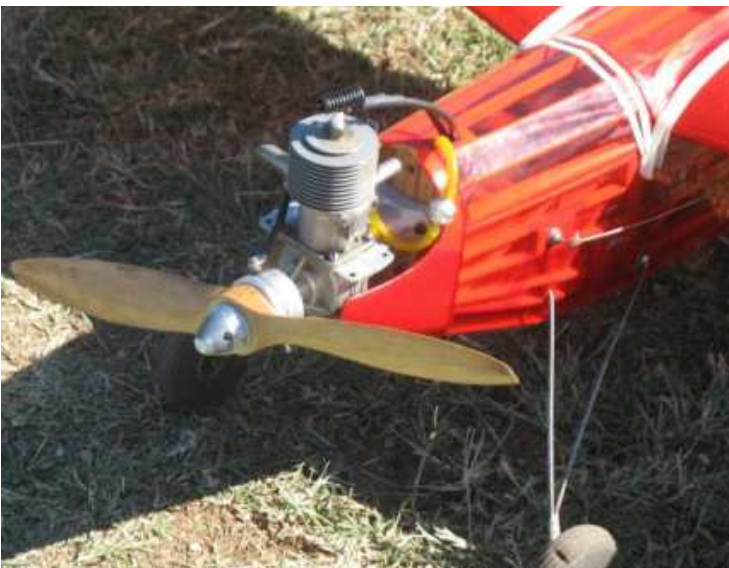
Forster 99 powered Cumulus on spark by Kevin Fryer. Engine well sorted out and a very smooth and reliable runner.
