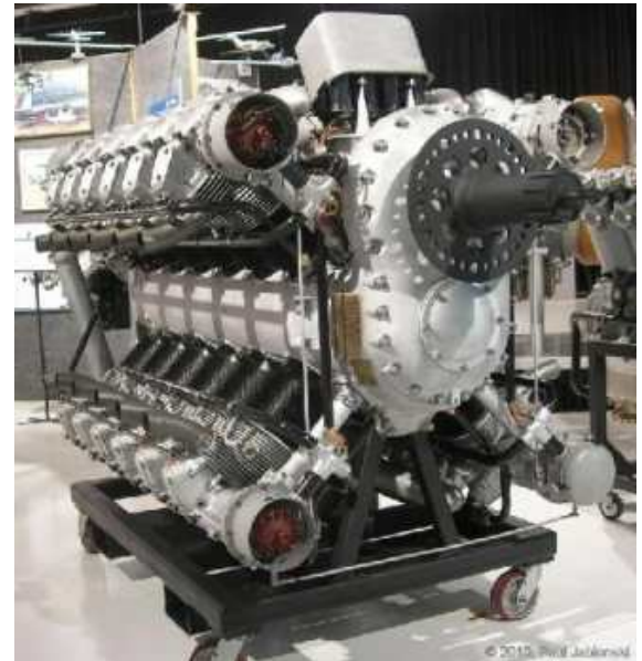
The restored Allison X-4520 24-cylinder, air-cooled engine carrying Allison serial number 1. Note the distributors on the front of each overhead camshaft. (Paul Jablonski image via the Aircraft Engine Historical Society)
