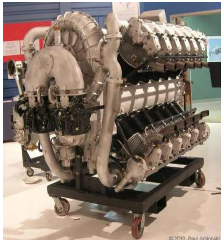
The Allison X-4520 on display at the Rolls-Royce Heritage Trust Allison Branch in Indianapolis, Indiana. Note the induction and how it differs from the 1925 drawing. (Paul Jablonski image via the Aircraft Engine Historical Society)
