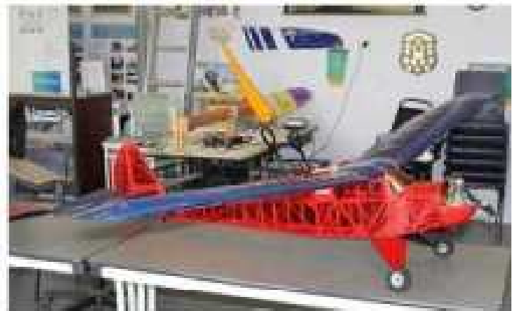
Trevor Boundy's "Westerner" a 1938 design by Elbert Weathers and powered by an open rocker OS60 four stroke engine.
