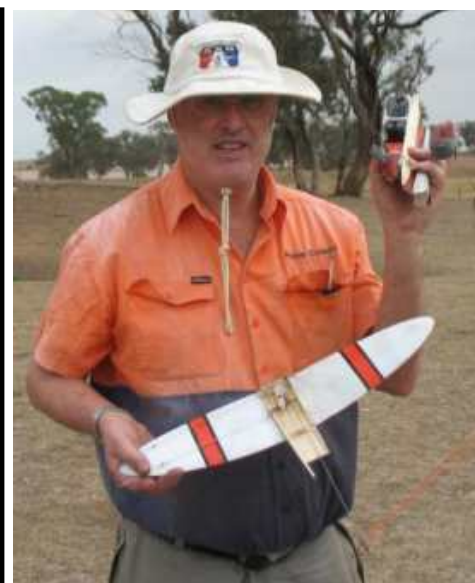
What happens when your Phantom goes too fast - wing parts company with fuselage which, complete with engine, is flung 30 metres across the paddock scaring the spectators. Bad luck Condo.
