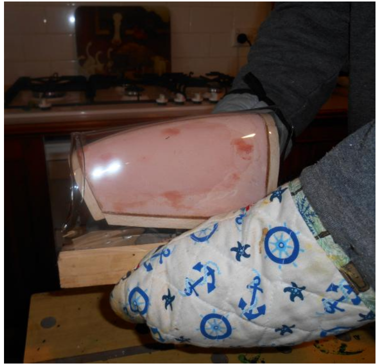
Moulding the canopy.
