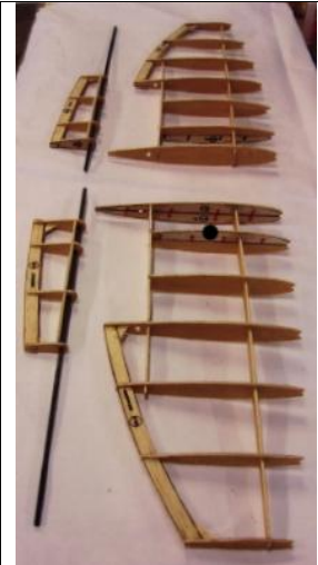
Very delicate wing, but carbon fibre rod as flap hinge.
