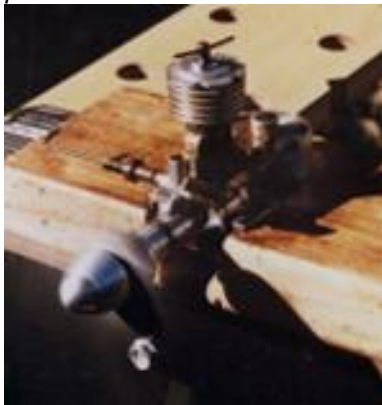
ED Mark 111 2.49cc Front rotary 1948 engine running nicely on APC 10x5 prop. Not easy starting
