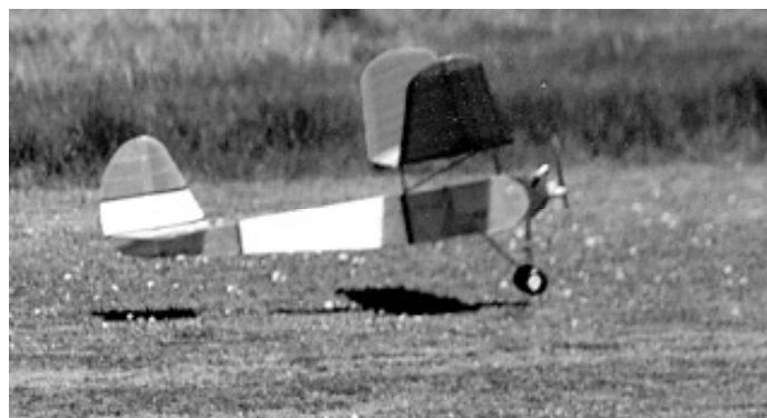
Lanzo Record Breaker, Saito 45, built 1989 by Allan Laycock, tissue covered.
