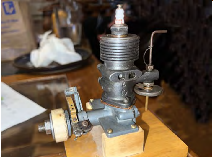
Sky Chief .526 cu. in. Ignition engine by Supercraft, Circa 1940.
