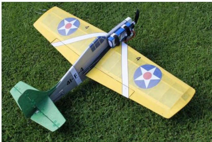
A Grumman Wildcat built by Tim Cooper for carrier competitions. The model is electric powered and uses radio control to work the throttle .
