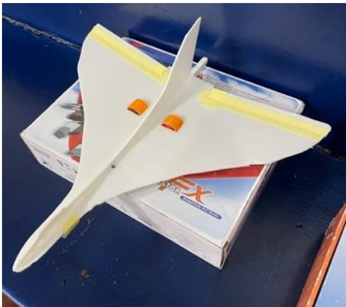
Greg Egan's own design Avro Vulcan. Photo on left is the model as originally set up with the electric fans embedded in the wings. Photo on the right shows the current arrangement with the motors mounted below the wings and a nose broken during trials. The masking tape is a convenient means of positioning the CG and modifying other items during the test flying stage. Motor mountings, shrouds and propellers are 3D printed by Greg.
