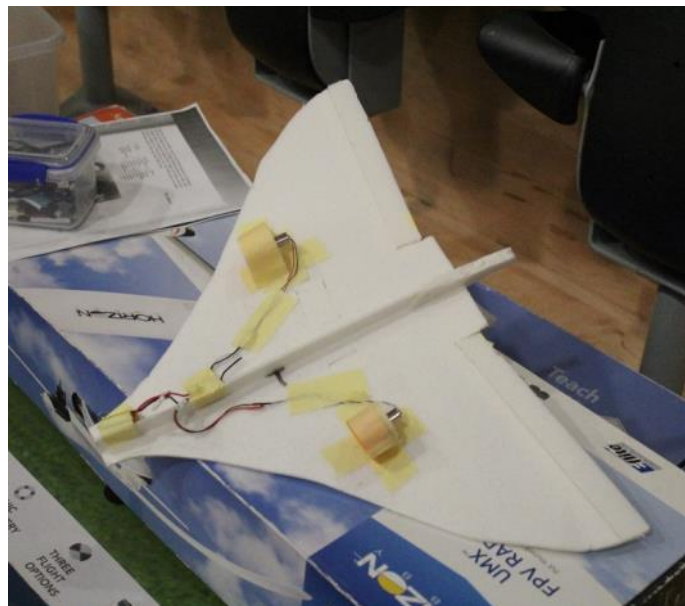
Greg Egan's own design Avro Vulcan. Photo on left is the model as originally set up with the electric fans embedded in the wings. Photo on the right shows the current arrangement with the motors mounted below the wings and a nose broken during trials. The masking tape is a convenient means of positioning the CG and modifying other items during the test flying stage. Motor mountings, shrouds and propellers are 3D printed by Greg.
