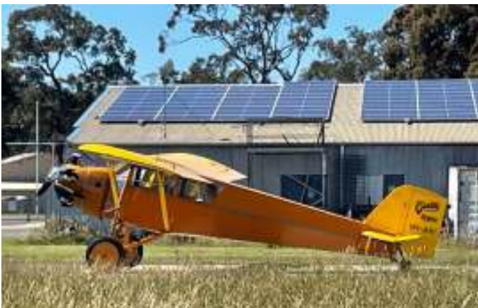
This Curtiss Robin Model B, owned by a resident of Patterson Lakes, Victoria, was recently photographed at the Traralgon airfield in Gippsland, Victoria. Powered by a Wright R-540 Whirlwind radial engine it's a rare bird.
