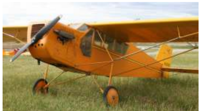
David's model of the Curtiss J-1 Robin with the Curtiss OX-5 90hp V-8 engine.
