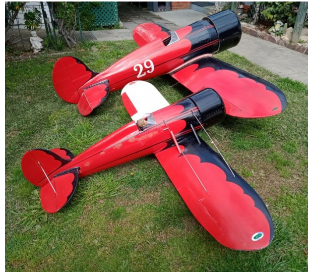
The 1.7m wingspan model built from the original plan together with the scaled up 3m version.
