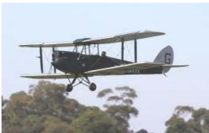
Rob Popelier's 1/4 scale DH60 Gipsy Moth flying in F4C. The model has a wing-span of 2.3m and is powered by an OS 120 four stroke engine,
