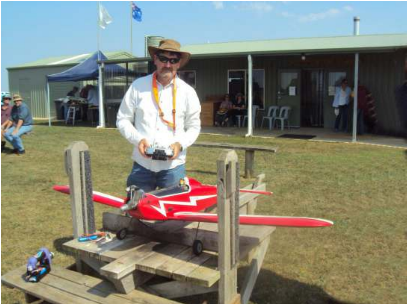
Bruce Thompson's 1.8m Astro Hog powered, by an OS 95 four stroke engine, was built from a SIG kit.
