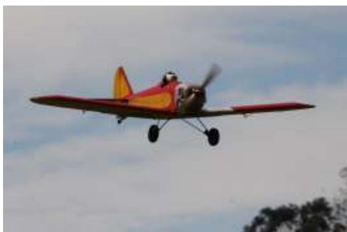
Lionel Carpenter's 1/4 scale Bowers Flybaby powered by a RCGF 20cc twin cylinder petrol engine.
