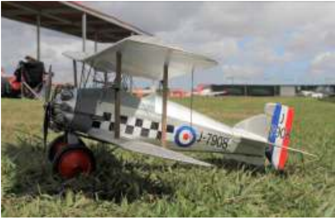
Roly Gaumann's scratch built Gloster Gamecock has a wingspan of 1.1m. The model is electric powered and was developed from an Aeromodeller plan for a free flight aircraft. Roly's other model is an ARF Boeing 737 Max with a wingspan of 2.0m and driven by two electric ducted fans.
