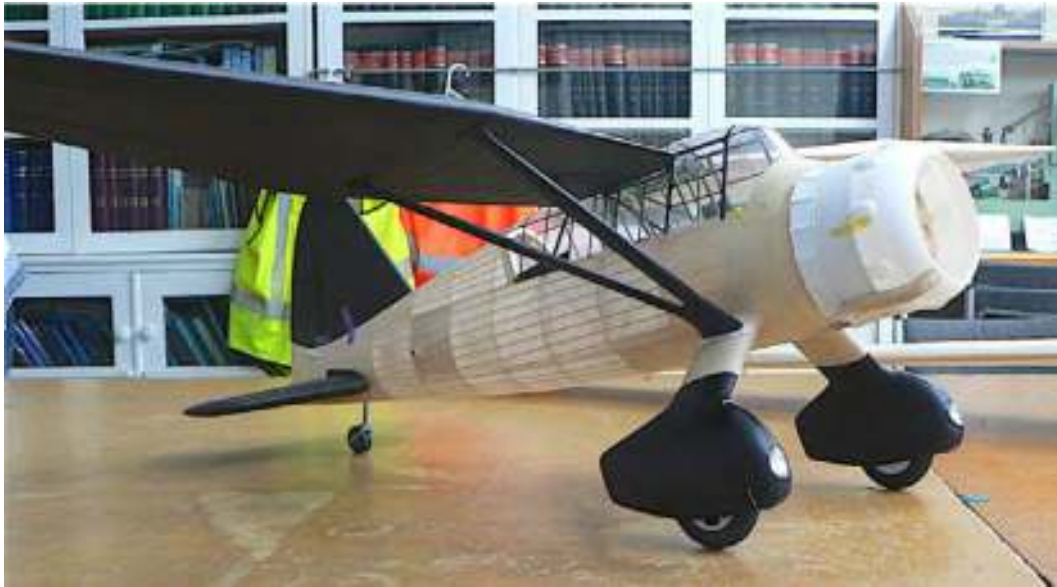
Mike Mulholland's rubber powered 1.27m wingspan Westland Lysander is nearing completion.
