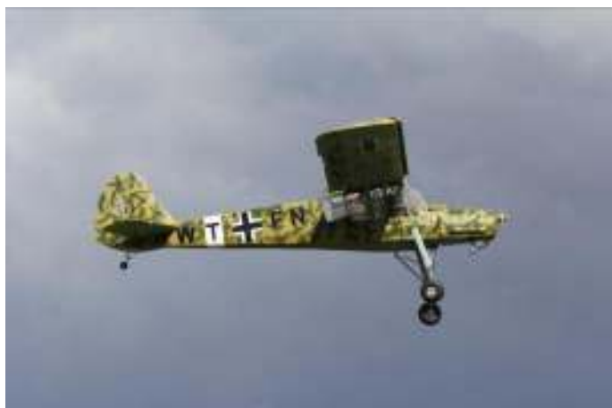
Brian Evans with his 1/4 scale Fieseler Fi-156 Storch. The scratch built model has a wingspan of 3.8, weighs 16kg and is powered by a DA50 petrol engine.
