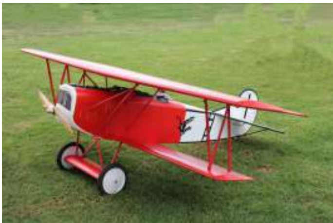
Rod Watkins' ARF 1/4 scale Fokker D.VII has a wingspan of 2.2m.
