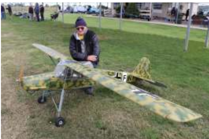
Brian Evans with his 1/4 scale Fieseler Fi-156 Storch. The scratch built model has a wingspan of 3.8, weighs 16kg and is powered by a DA50 petrol engine.
