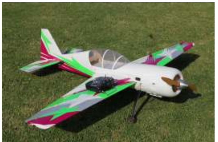
Lionel Carpenter's ARF Yak-54 powered by a DLE 35 petrol engine.
