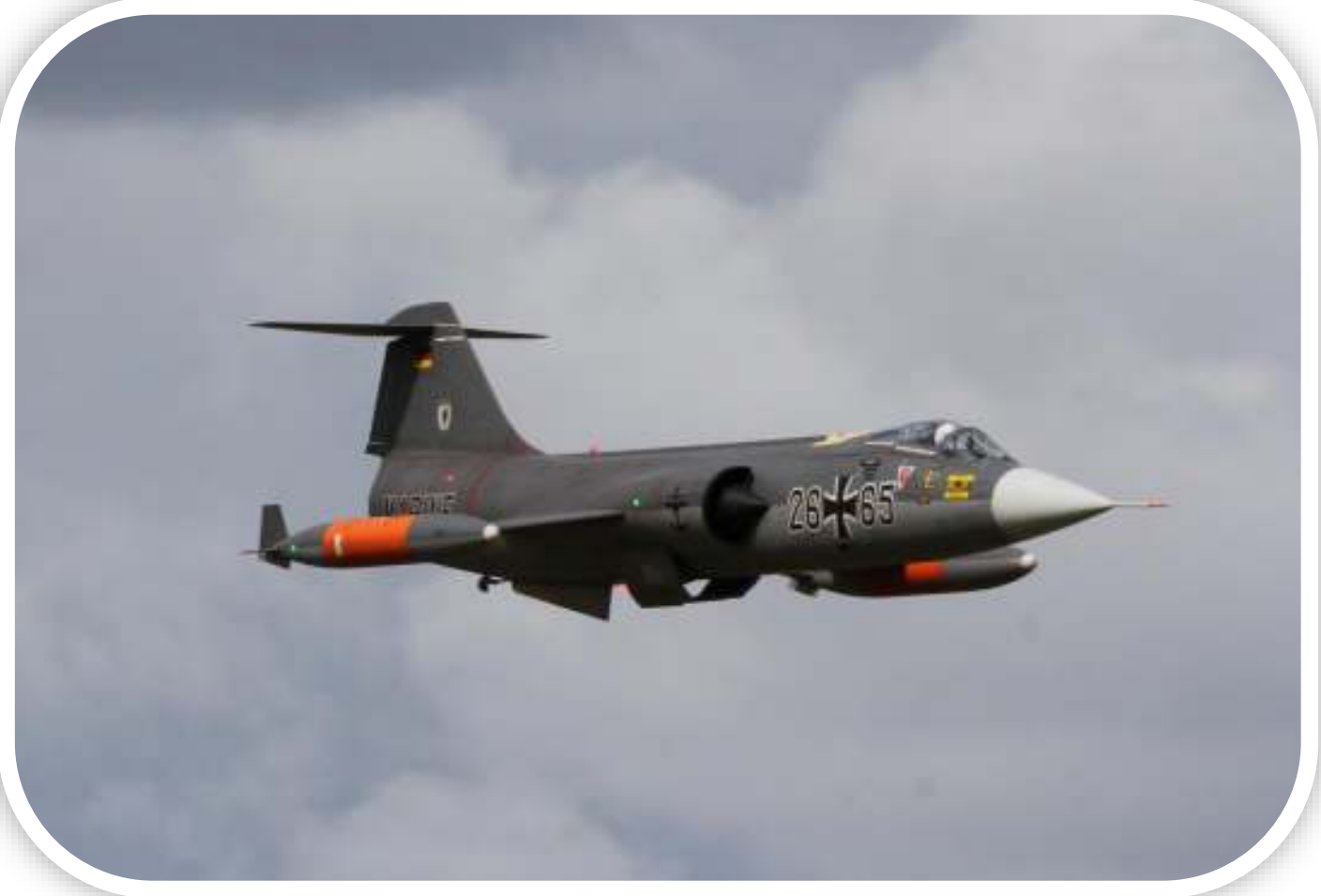
Steve Wilcox's ARF 1/4 scale F-104 Starfighter is powered by a Jetcat P300 turbine delivering 67kg of thrust. It was a spectacular sight with its size and performance and provided the highlight of the event.
