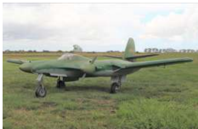
Rod Mitchell's scratch built McDonnell XP-67 Moonbat is 2.54m wingspan and powered by two OS 91 two stroke engines.
