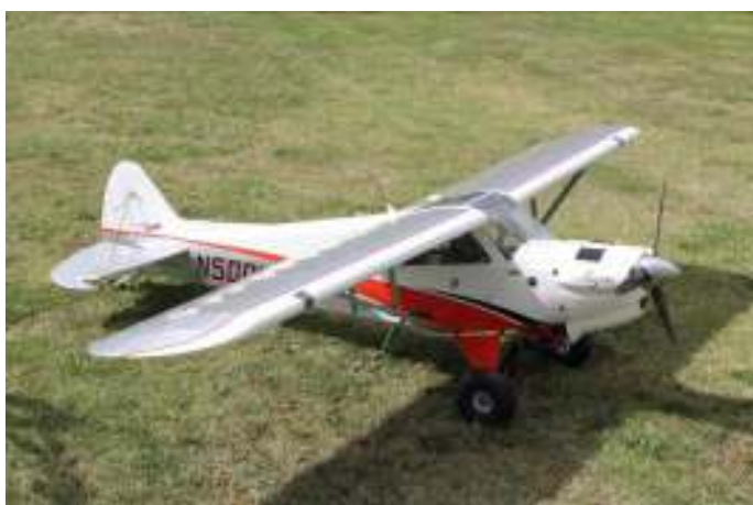
Adam Barker's 1/3 scale XCub, an ARF by Hangar 9 is 2.93m wingspan and weighs 14.1kg. The model is powered by a DLE 60cc twin cylinder petrol engine.
