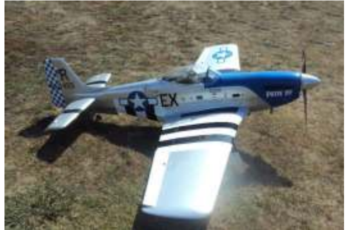
Bruce Thompson's Phoenix ARF P-51 Mustang. The model is 2.2m wingspan and is powered by an OS 60cc two stroke petrol engine. Bruce has raced the Mustang in Adelaide.
