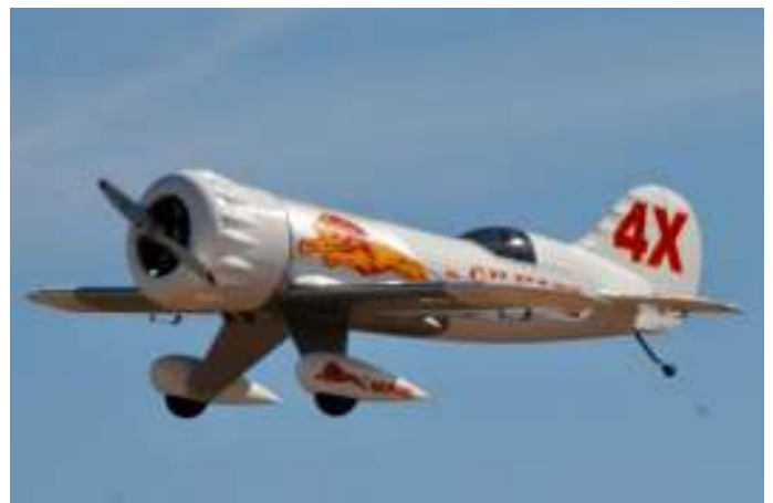
Wedell Williams 'Gilmore' racer owned by Graeme Cashman and piloted by Wes Wright. This model is 1/3 scale and powered by a Valach 250 engine.
