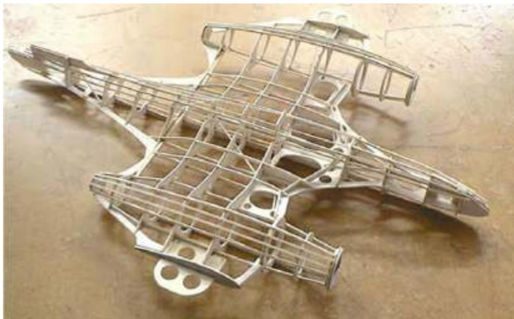
Don Spray's rubber powered McDonnell XP-67 Moonbat is progressing. Covering will be an interesting exercise.
