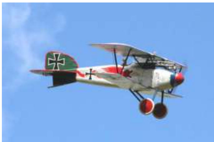
Ian Farrar's Albatros D.III has a wingspan of 2.25m and was scratch built from the Gary Sunderland plan. Powered by a NGH 38cc petrol engine the Albatros re-uses the wheels, spinner and radiator from Gary's model.
