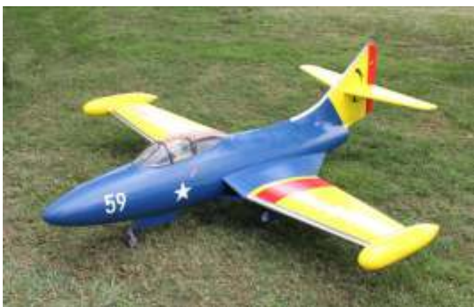
Rod Mitchell's Grumman Panther is 1.8m wingspan and powered by a Kingtech 80 turbine.
