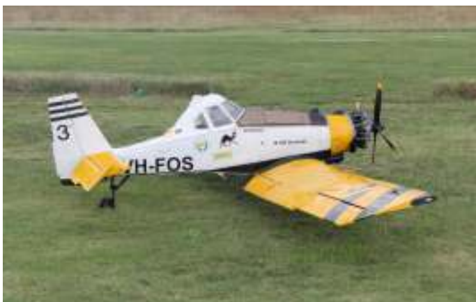
David Chivers' scratch built, 1/4 scale model of the Polish PZL-M18 Dromader-crop duster. The model weighs 56kg and is powered by a Moki seven cylinder, four stroke, radial engine.
