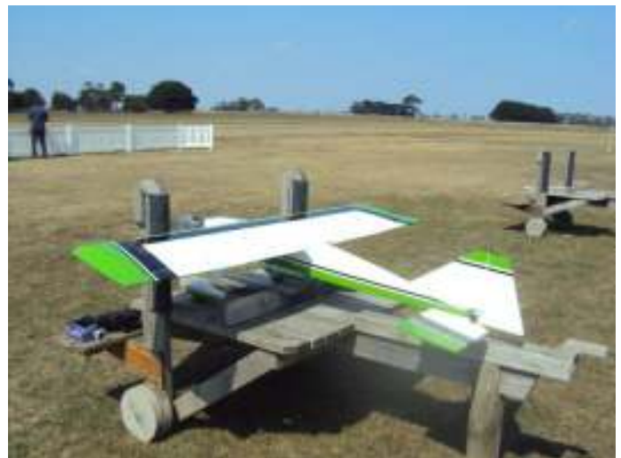
Bruce Thompson's Phoenix ARF P-51 Mustang. The model is 2.2m wingspan and is powered by an OS 60cc two stroke petrol engine. Bruce has raced the Mustang in Adelaide.
