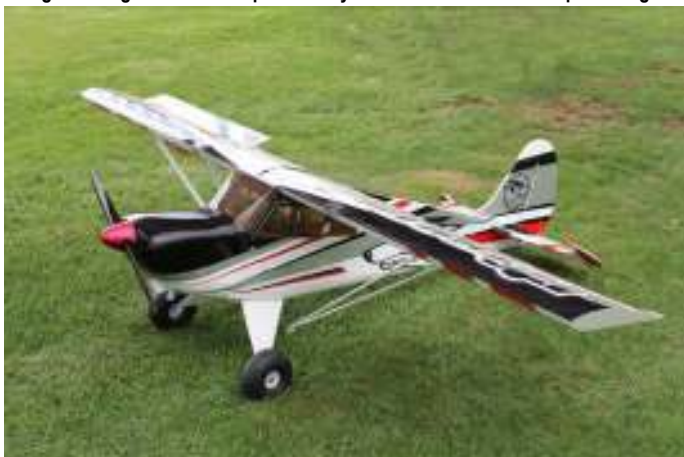
Adam Barker's 1/3 scale XCub, an ARF by Hangar 9 is 2.93m wingspan and weighs 14.1kg. The model is powered by a DLE 60cc twin cylinder petrol engine.
