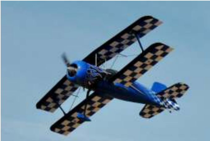
Pitts 12 powered by a Moki 250 and flown by Wes Wright from Eden, NSW.
