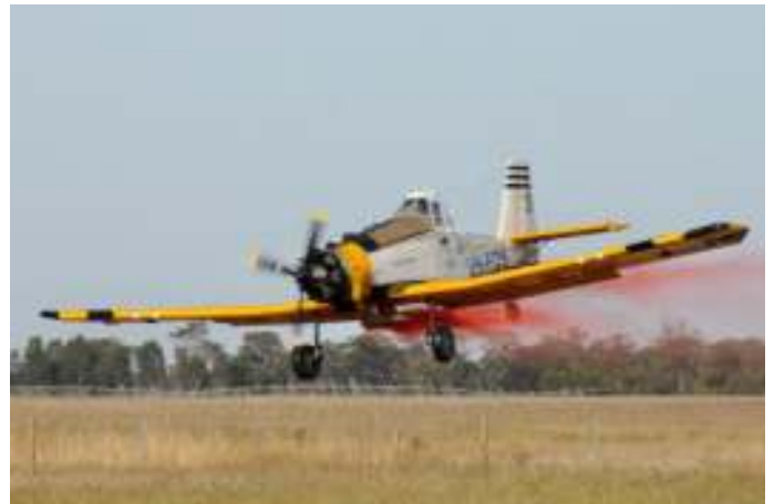
Dave Chivers' Dromader powered by a Moki 350 engine, on a fire bombing run.
