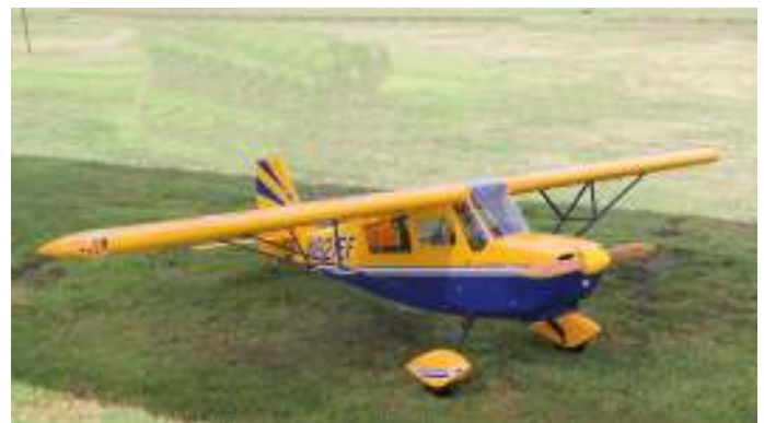
Richard Wiggan's Seagull ARF Super Decathlon has a wingspan of 3.1m, weighs 13kg and is electric powered.
