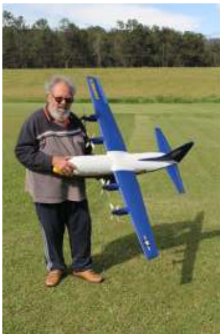
Peter Wyatt with his Avios ARF Hercules C-130J . The foam model spans 1.6m and is electric powered.
