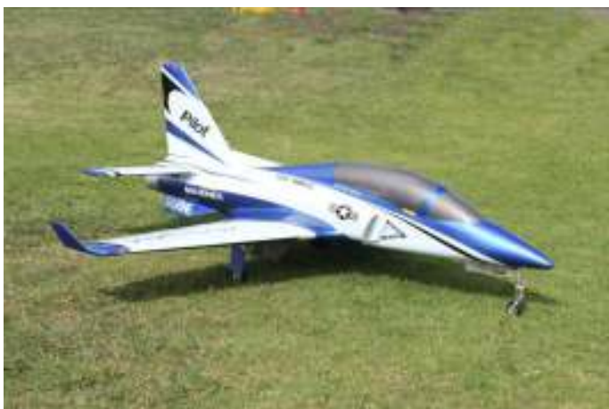
Richard Wiggan's Phoenix ARF Tucano T-27 has a wingspan of 2.6m, is electric powered and weighs 11kg.
