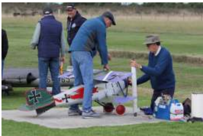
Ian Farrar's Albatros D.III has a wingspan of 2.25m and was scratch built from the Gary Sunderland plan. Powered by a NGH 38cc petrol engine the Albatros re-uses the wheels, spinner and radiator from Gary's model.
