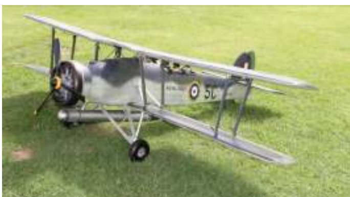
Peter Mack's ARF Fairey Swordfish by ESM has a wingspan of 2.1m, weighs 12kg and is electric powered.
