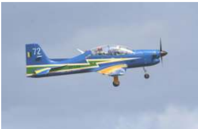
Richard Wiggan's Phoenix ARF Tucano T-27 has a wingspan of 2.6m, is electric powered and weighs 11kg.
