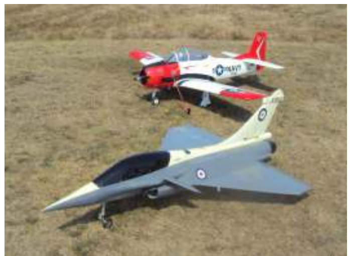
Ric Pimblott's 2.00m E-Flite Trojan powered by a brushless 70mAh motor with his 1.14m wingspan ARF Rafael powered by a Kingtech 80 turbine and weighing 7.5kg. Both models use Hitec HS645 servos.
