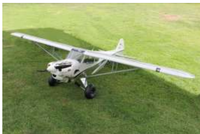
Keith Quigg's 1/3 scale XCub, an ARF by CubCrafters, is 3m wingspan and weighs 13kg. The model is powered by a DLE 55cc petrol engine.
