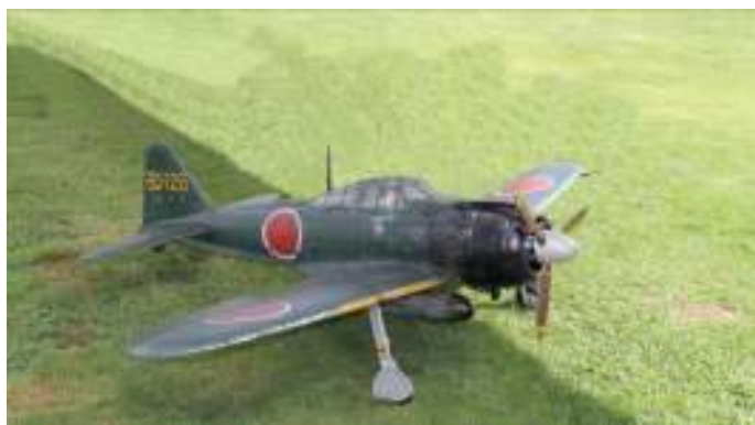
Peter Mack's ARF A6M5 Zero by Top RC has a wingspan of 2.3m and weighs 15kg. The model is powered by a Saito 90cc four stroke petrol engine.
