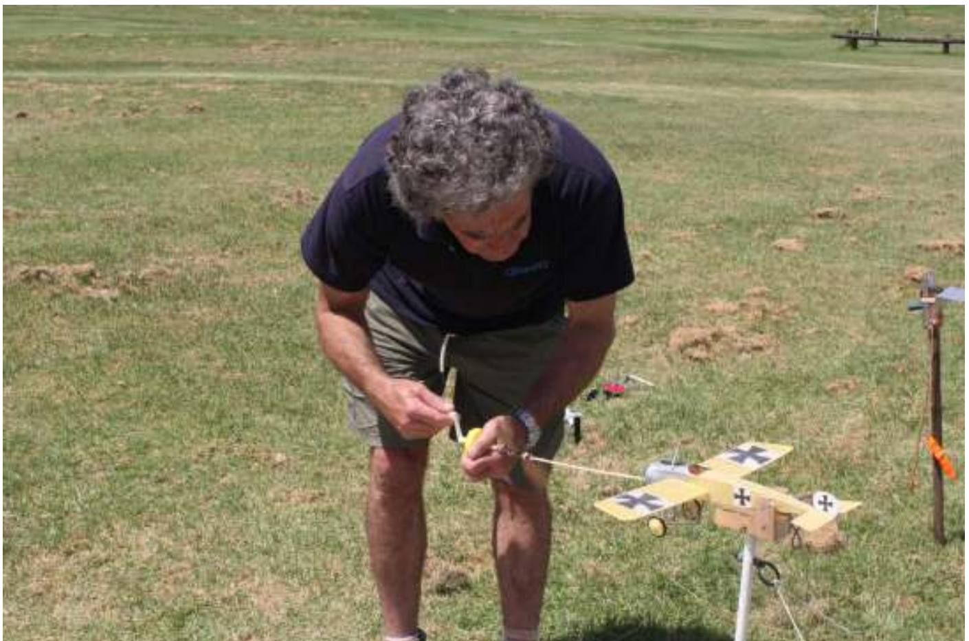
Tim Cooper winding the rubber motor in his Peanut Scale Fokker E.III. Peanut Scale models are an indoor model class and are limited to 330mm wingspan. They may have little or no dihedral, depending on adherence to the design of the full sized aircraft, so dead calm conditions are required for successful outdoor flying.
