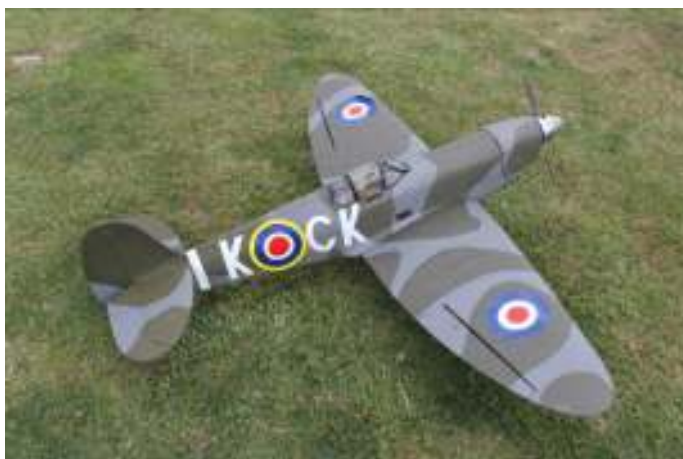
David Nicholls Spitfire is an ARF by Sportsman Aviation. The model has a wingspan of 1.6m and is powered by an ASP 91 four stroke engine.
