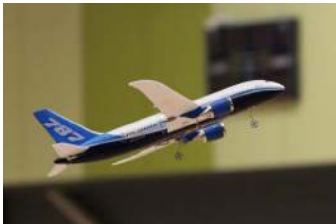
Ron Van Bemel's Boeing 787 is from Banggood. The model is 550mm wingspan with elevators for pitch control and two ducted fans for thrust and yaw control.
