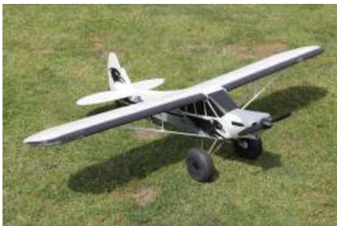
Graham Jenner's Super Piper Cub is a 1/6 scale foam ARF with a wingspan of 1.7m.
