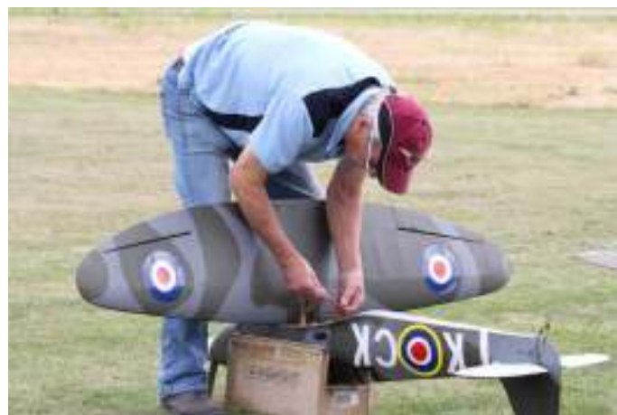
David Nicholls Spitfire is an ARF by Sportsman Aviation. The model has a wingspan of 1.6m and is powered by an ASP 91 four stroke engine.
