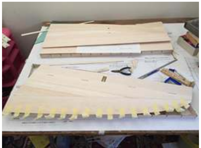
The top sheeting was held in place with masking tape while the glue dried.
