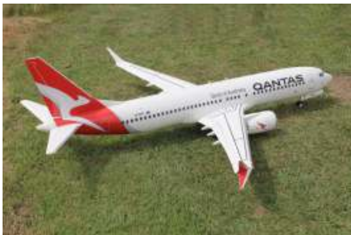
Peter Feller's Boeing 737 is a foam ARF powered by two 70mm diameter electric ducted fans.
