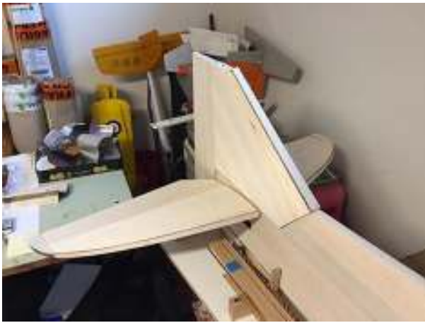
The tailplane is all moving, pivoting on a carbon tube.
