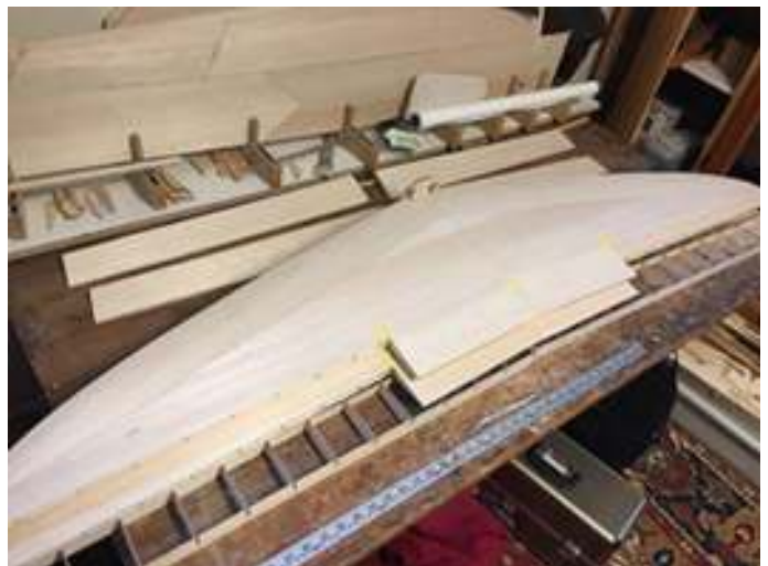
Anhedral is added by placing a piece of wood under the centre of the cradles as the panels are joined.
