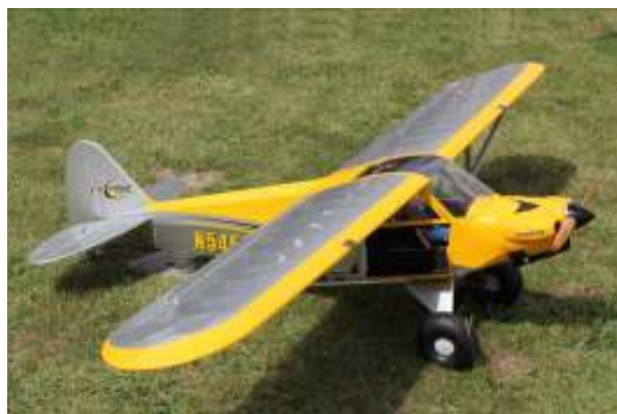
Peter Feller's ARF Hangar 9 Carbon Cub. This model is 1/5 scale, 2.29m wingspan and powered by a DLE 20 petrol engine. The Cub is very well finished as are most Hangar 9 models.
