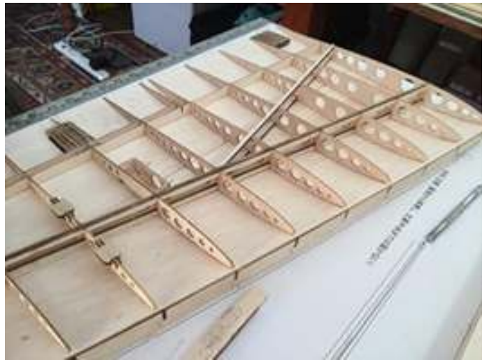
Look at all that lightness! The ailerons are cut from the wing panels once they are completed.
