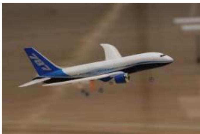
Ron Van Bemel's Boeing 787 is from Banggood. The model is 550mm wingspan with elevators for pitch control and two ducted fans for thrust and yaw control.
