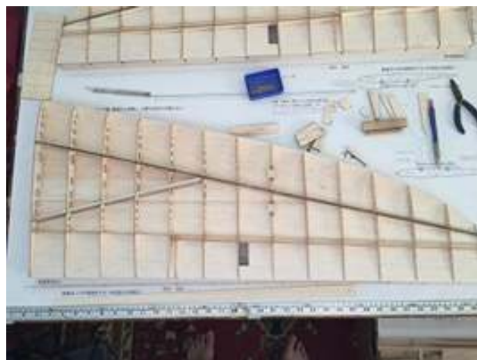
Anhedral is added by placing a piece of wood under the centre of the cradles as the panels are joined.
