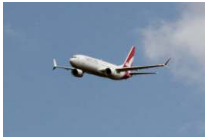
Peter Feller's Boeing 737 is a foam ARF powered by two 70mm diameter electric ducted fans.
