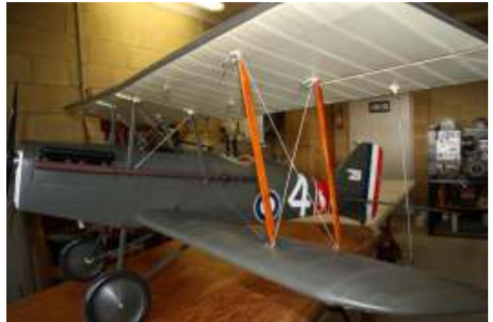
Stainless steel rigging wires replaced the hat elastic of the kit.
