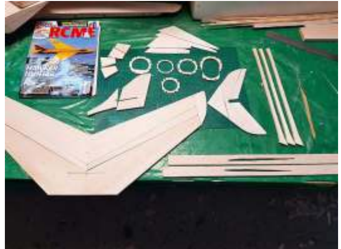
The Hunter has a planked fuselage with sheet balsa flying surfaces.
