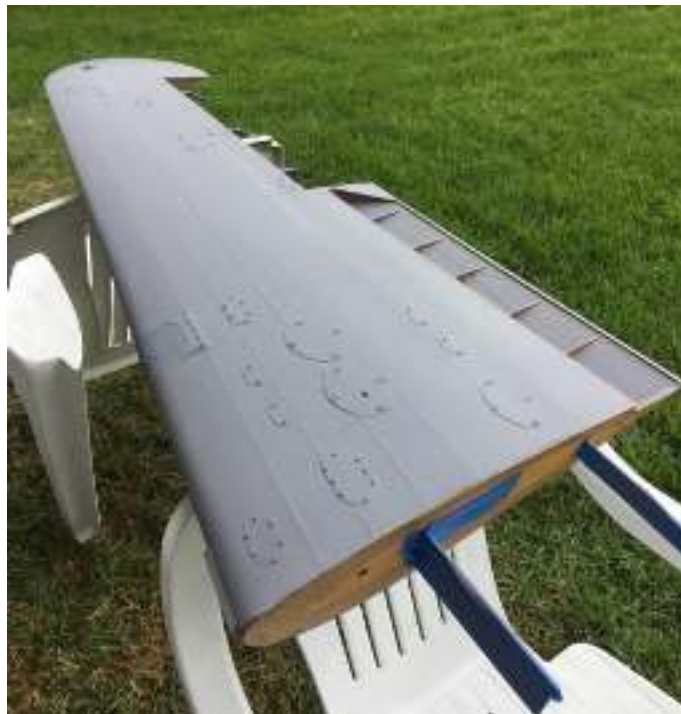
The underside of the lithoplated port wing outer panel with access covers.
