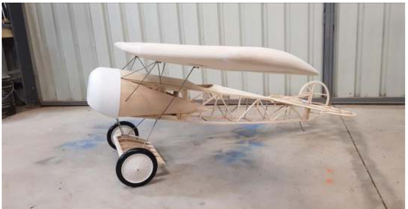
The base structure of Tim's Fokker D.VIII ready for covering.
