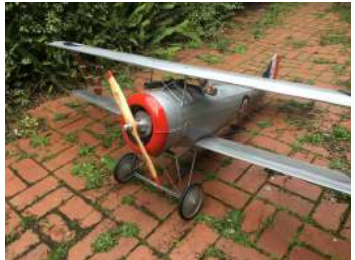
Haydn's 1/4 scale Nieuport 27 is scratch built from plans by the late Gary Sunderland and powered by a copy of a Honda 36cc four stroke engine.
