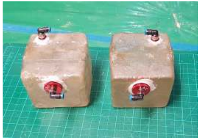
Custom built fiberglass fuel tanks to suit the engine nacelles.
