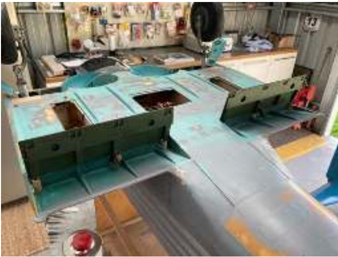
Underside of wing centre section showing the flaps and access to radio gear.
