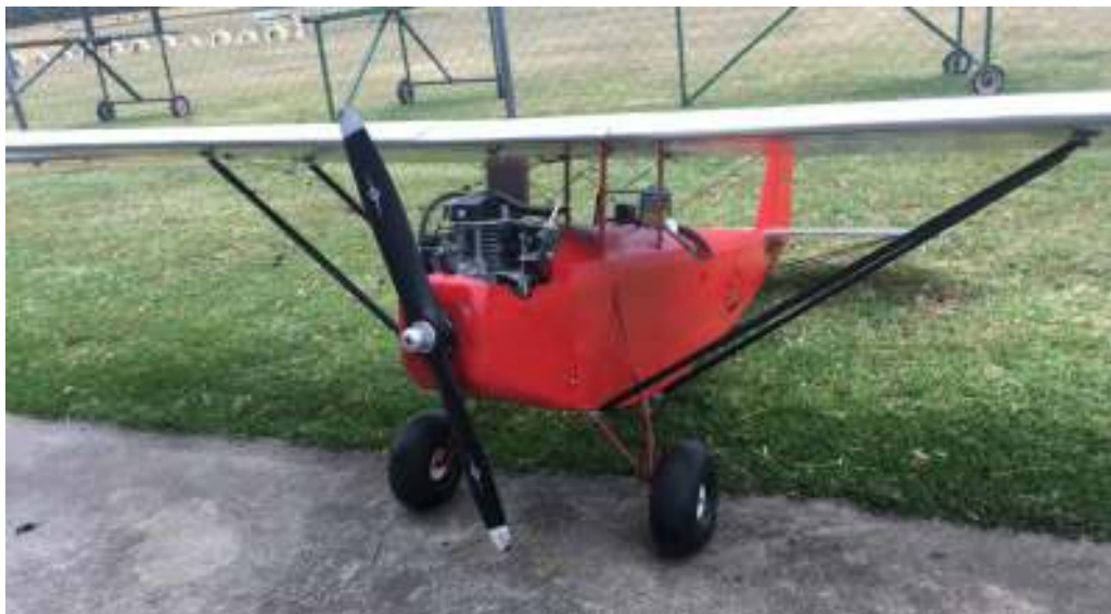
The 1/3 scale Pietenpol Air Camper is powered by a modified 32cc brush cutter engine.
