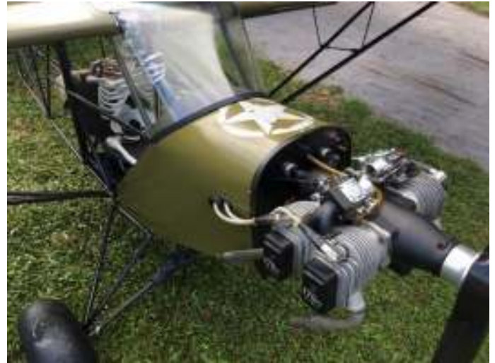
Fellow Port Macquarie member Doug Way's Scrub Cub is powered by a Roto 170 four cylinder four-stroke petrol engine.
