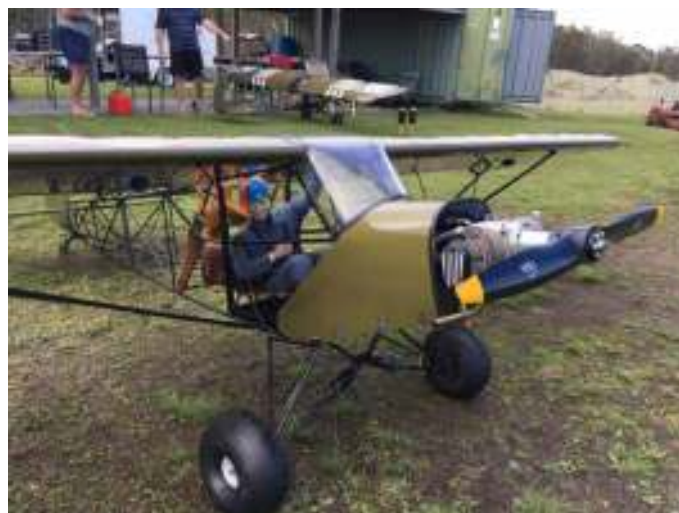
Mike's Scrub Cub is powered by a twin cylinder four-stroke engine.
