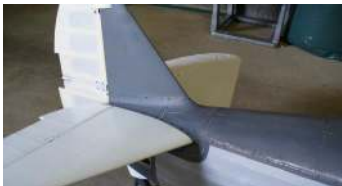
Lithoplate fairings on the rear deck and fin.
