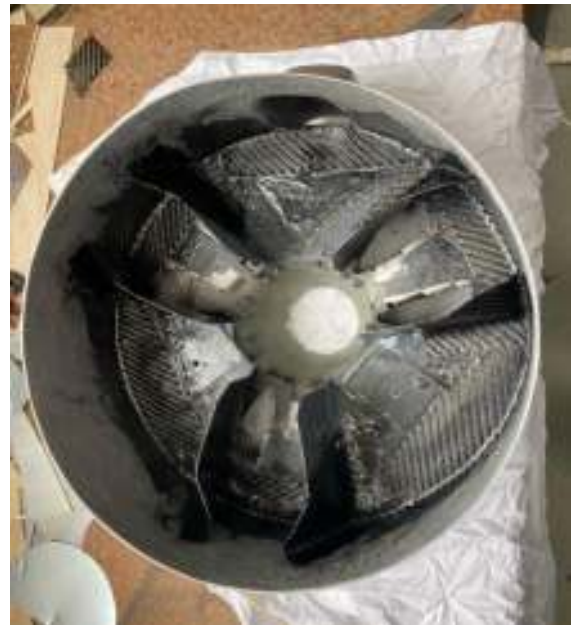
Fibreglass baffles direct cooling air over the Saito 90cc engine.
