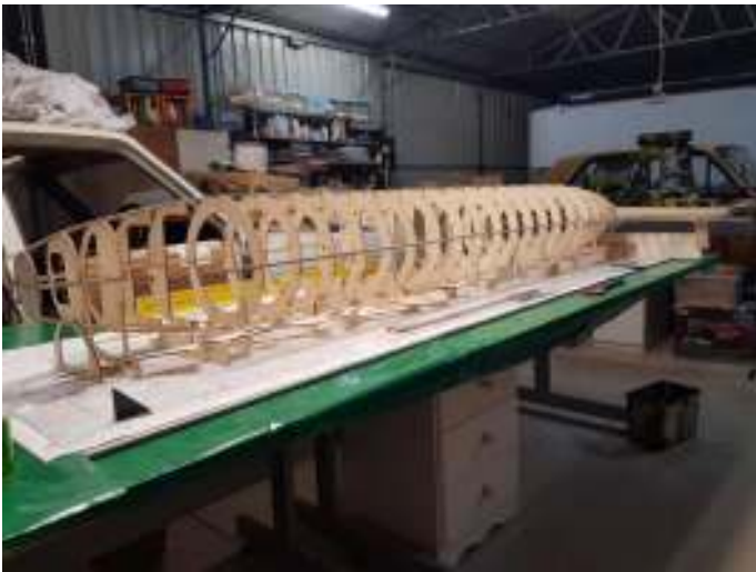
Fuselage framework in progress.
