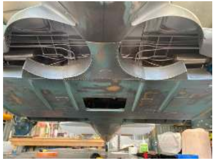
Wheel wells with detailed hydraulic tubing.
