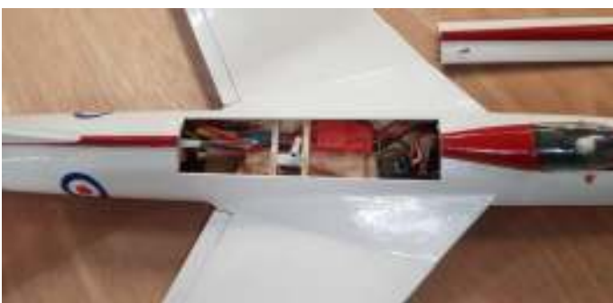
Radio, servos and fan are accessible through a top hatch.
