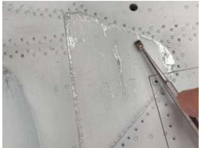
Simulated weathering applied to the aluminium panels.
