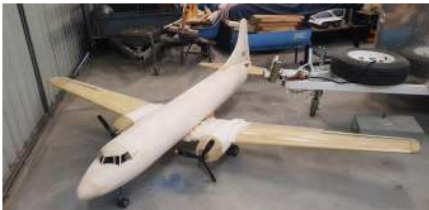
The present state of construction with the Convair. Almost ready for the fuselage and wing centre section to be fibreglassed.
