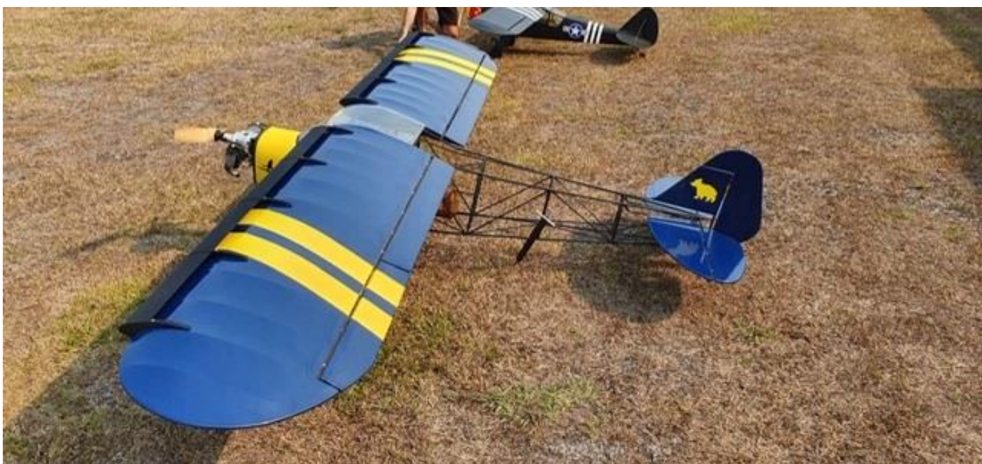
A Scrub Cub fitted with leading edge slats for even greater STOL performance.
