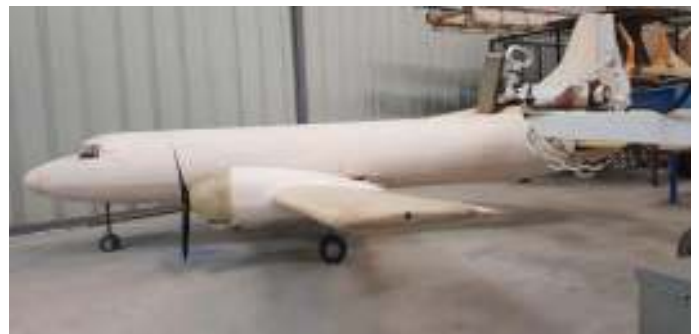
The present state of construction with the Convair. Almost ready for the fuselage and wing centre section to be fibreglassed.
