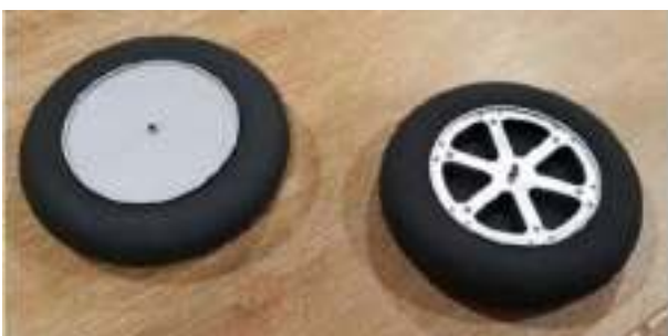
Wheels finished and painted weigh 6g each.
