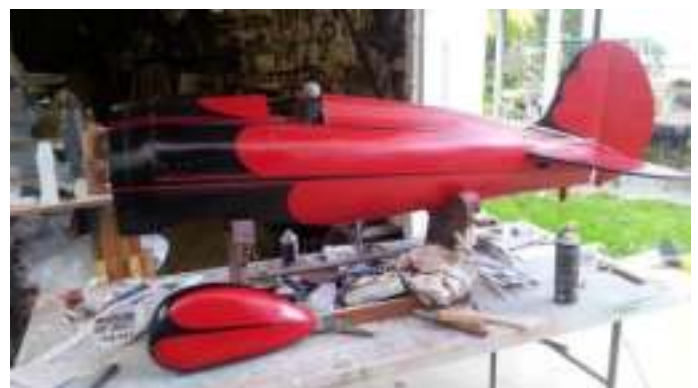
Fuselage and wings are fully sheeted, wheel pants are carved from high density foam.
