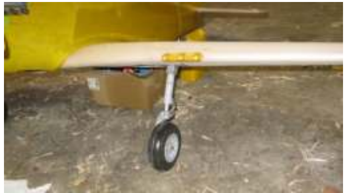
The retracting undercarriage is also designed and built by Glen.
