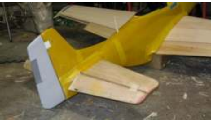
Glen started his Mustang build 15 years ago and has now resumed construction. The model is 1/5 scale with a wingspan of 2.29m and is scratch built, including the plug and mould for the fibreglass fuselage.
