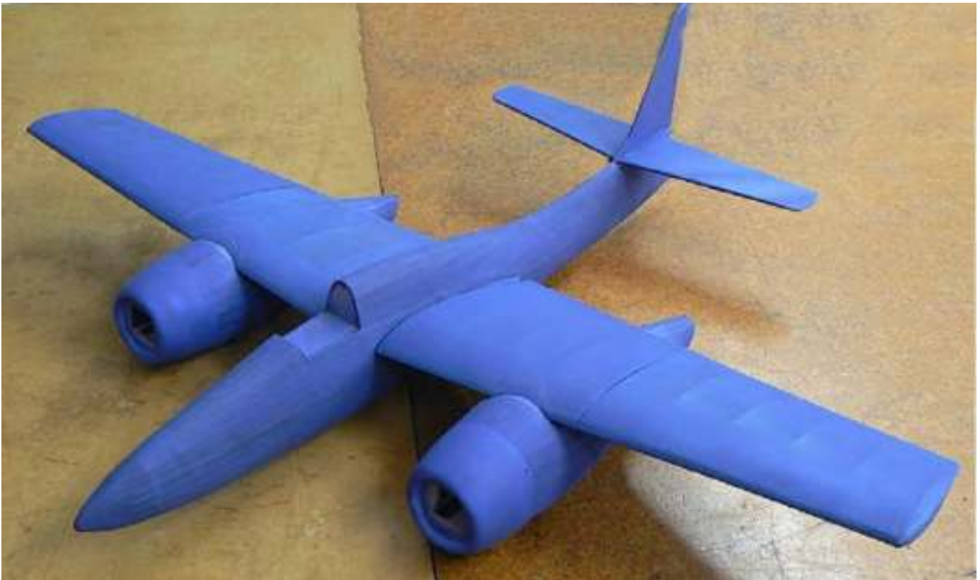
The 1m wingspan, rubber powered Tigercat covered and ready for propellers, canopy and markings.
