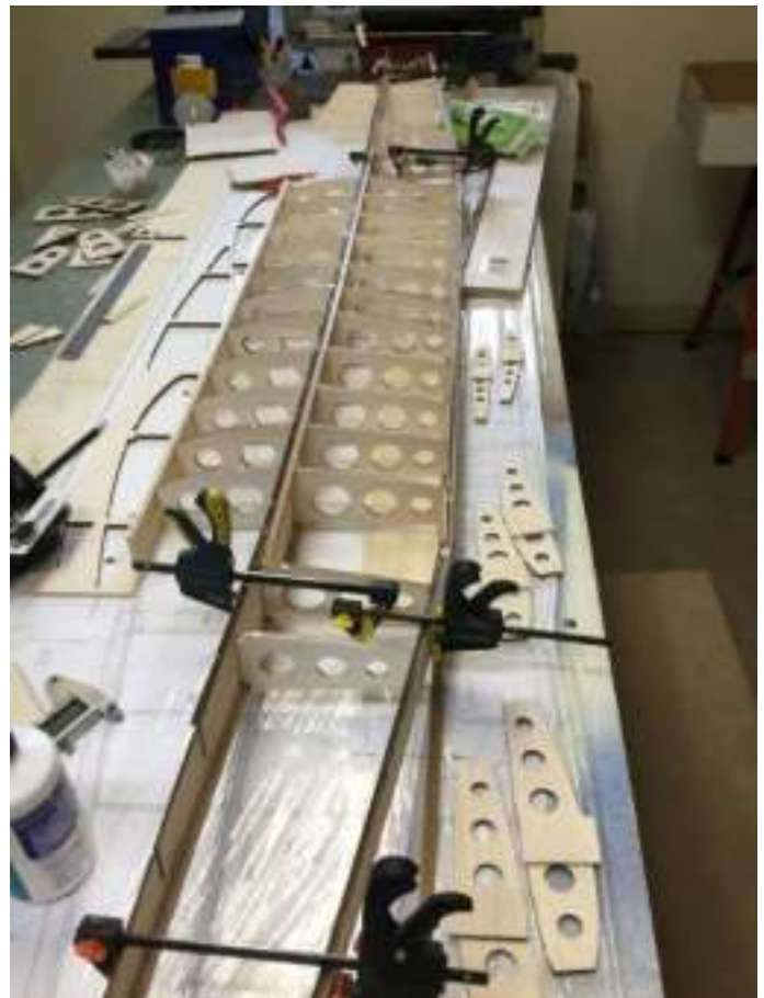
Wing construction, clamps are always handy.
