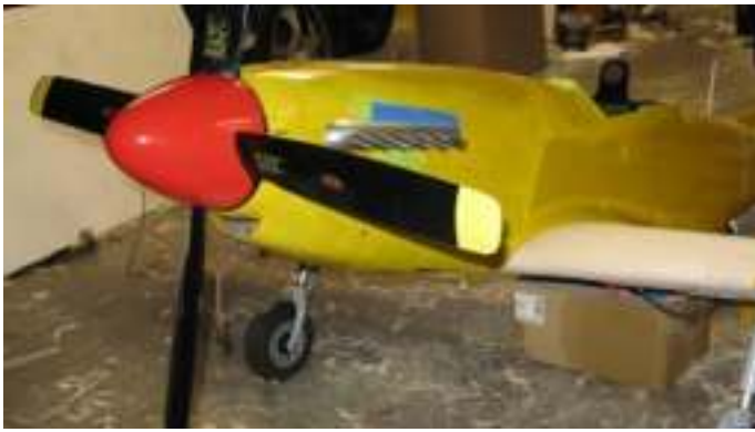
The Mustang is powered by a 3W 70cc petrol engine.
