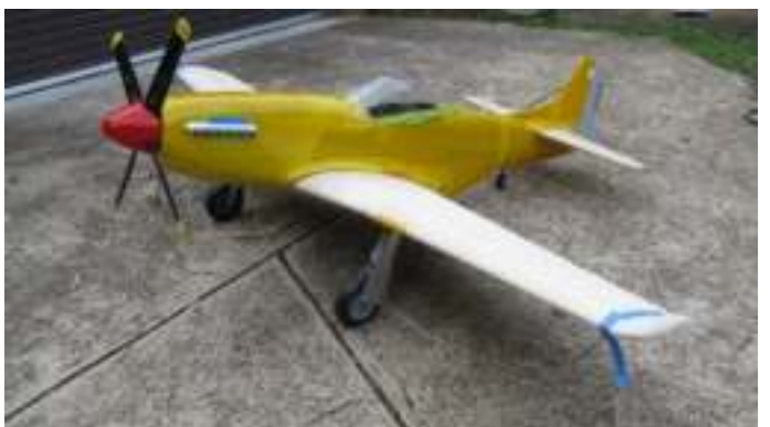
Glen started his Mustang build 15 years ago and has now resumed construction. The model is 1/5 scale with a wingspan of 2.29m and is scratch built, including the plug and mould for the fibreglass fuselage.
