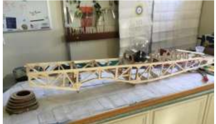
Assembly of the basic fuselage box.
