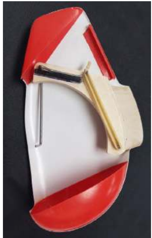
Vacuum formed wheel pants.
