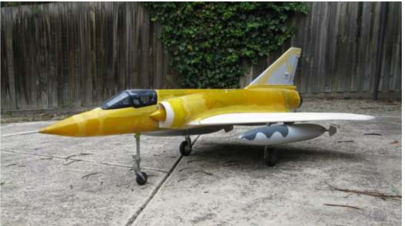
Glen's Mirage III is scratch built to 1/6 scale with a fibreglass fuselage and balsawood wing. Construction started 20 years ago and the Covid 19 lockdown has provided the impetus to get him back at work on the model. The fuselage is 2.13m long and again the plug and mould were constructed by Glen. The model is powered by a Jetcat turbine producing 10kg of thrust.
