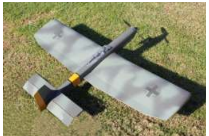
David Nobes built this 1.27m wingspan Ju.87 Stuka while in lockdown. The model performs well without flaps and is powered by an OS 25LA.
