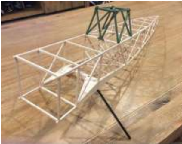
The basic fuselage box with the undercarriage mounting and scale wing mounting pylon.
