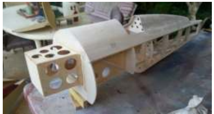
Construction is conventional balsawood / plywood.
