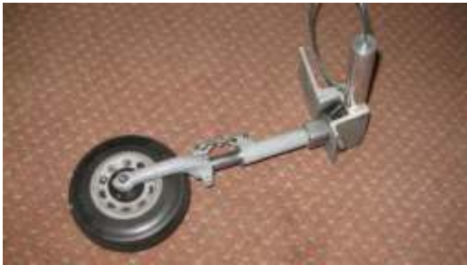
The retracting undercarriage is also designed and built by Glen.
