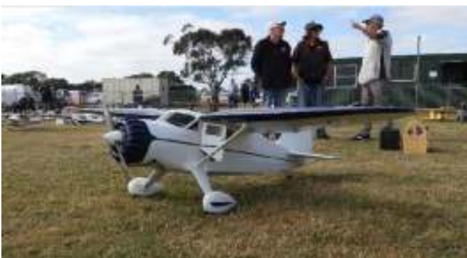
Robert Lauder's Stinson Reliant built from the Top Flite kit has a wingspan of 2.55m and is powered by an OS 40cc four stroke petrol engine .
