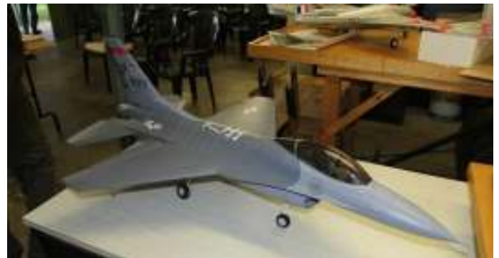
Cliff McIver's ARF foamy of the General Dynamics F-16 Fighting Falcon, powered by an electric ducted fan.
