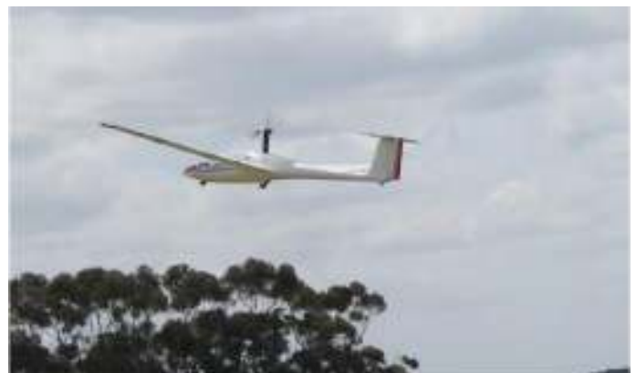
The ASK-21 glider on take-off flown by David Bell. The pylon mounted Hacker 60 electric motor had plenty of power.
