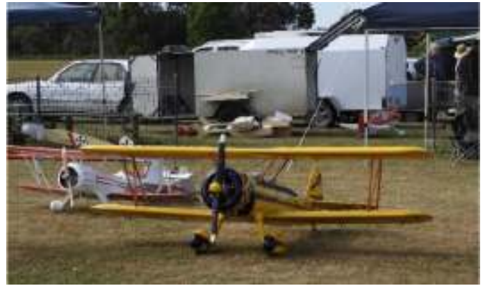
Garry Bergen's 1/3 scale Super Stearman built from a Balsa USA kit and powered by a Moki 215cc five cylinder, four stroke, radial engine.
