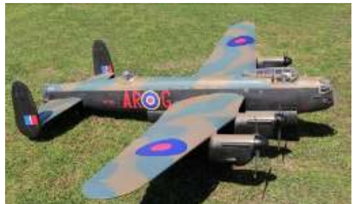
Ron Clark's scratch built Lancaster spans 3.4m and is powered by four Saito FG21 engines.
