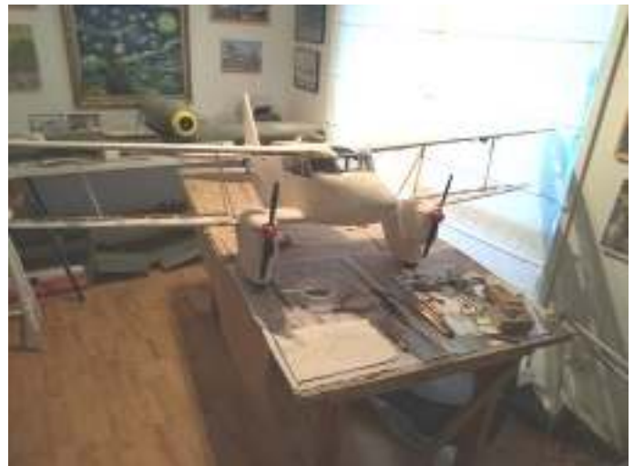
Norm Barclay's DH.90 Dragonfly nearing completion. The model spans 2m and is powered by two OS 29 two stroke engines
