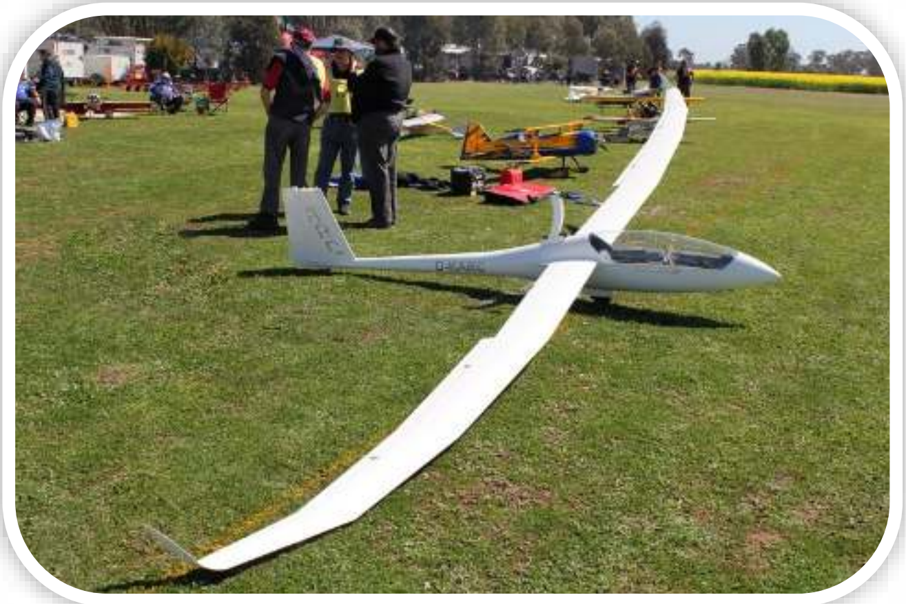
Jim Houdalakis' "Arcus" glider is an ARF manufactured in Czechoslovakia by H Models. The model is 40% scale with a wingspan of 8m and has an electric motor for self launching.
