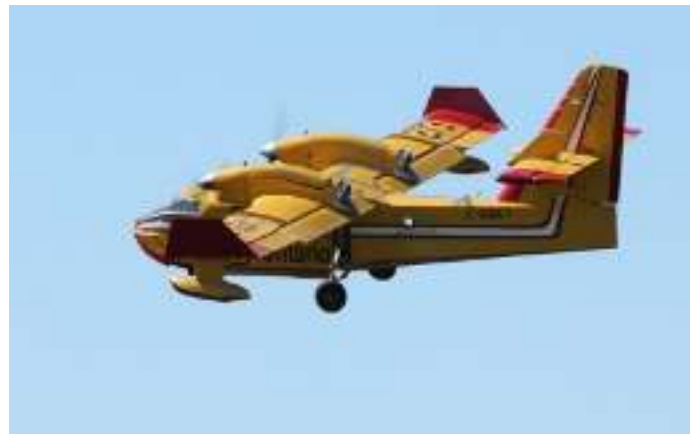
David Chiver's ARF Canadair CL-415 water bomber by MR Aerodesigns is 1/13 scale with a wingspan of 2.1m . The model is powered by two 46 AX OS two strokes and weighs 7kg.
