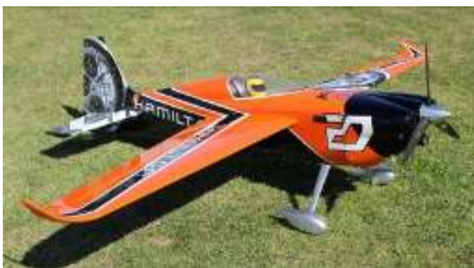
Keith Quigg's Pilot ARF Edge 540 is powered by a DLE 60 twin cylinder petrol engine and placed third in the Flying Only event.
