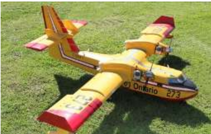
David Chiver's ARF Canadair CL-415 water bomber by MR Aerodesigns is 1/13 scale with a wingspan of 2.1m . The model is powered by two 46 AX OS two strokes and weighs 7kg.
