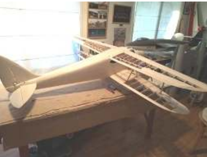
Norm Barclay's DH.90 Dragonfly nearing completion. The model spans 2m and is powered by two OS 29 two stroke engines
