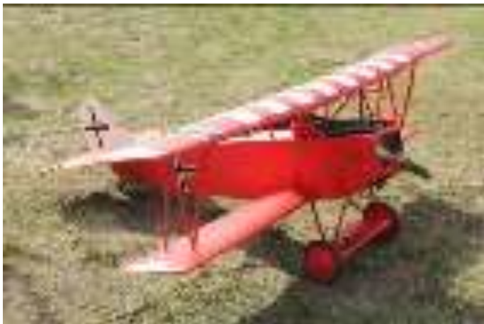
This 1/4 scale Fokker D.VII was built by Brett Cadwallader of the ACT from a Balsa USA kit and is powered by a Moki 210 two stroke engine.
