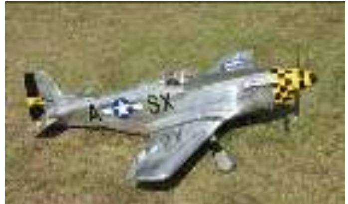
Tim De Haan's P- 51 Mustang is from a Topflite kit and is covered with aluminium Flitemetal. The model is 1/7 scale with a wingspan of 1.65m and is powered by an OS GT15 petrol engine.
