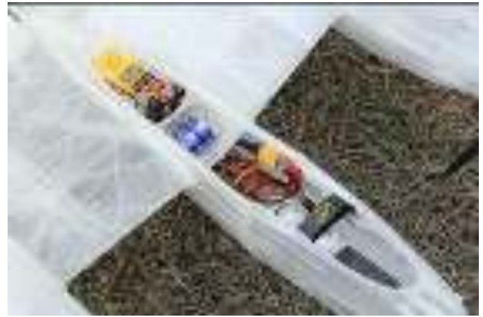
This Lockheed P-38 Lightning was produced by TCMAC member Tom Clark on a 3D printer. Forming in sections of 125mm length took a total of 100hrs and the sections were then joined to make an aircraft of 1.4m wingspan. Electric powered, it's a little heavy at 2.2kg but still flies well.
