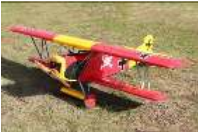
A 1/4 scale Hangar 9 ARF Fokker D.VII by Andrew Dore of the ACT. The model is powered by a Moki 50cc four stroke petrol engine.
