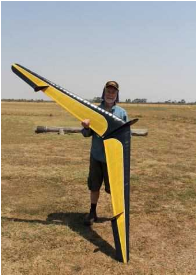
Trevor Boundy with his 1940 design "Sailwing" flying wing glider. The model is twice original size at 2.54m wingspan.
