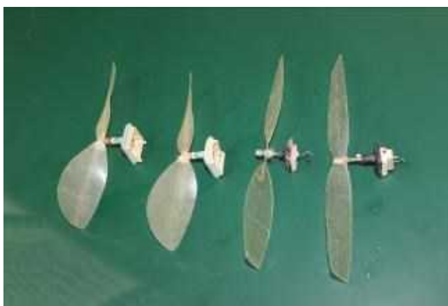
A range of superlight fibreglass props by Otto Haas.
