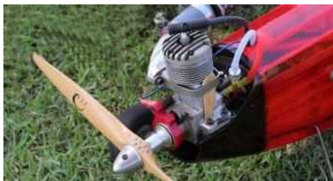
Close up of the reproduction McCoy 60 in Kevin Fryer's "Cumulus". The ice cream stick is a critical part of the exhaust system.
