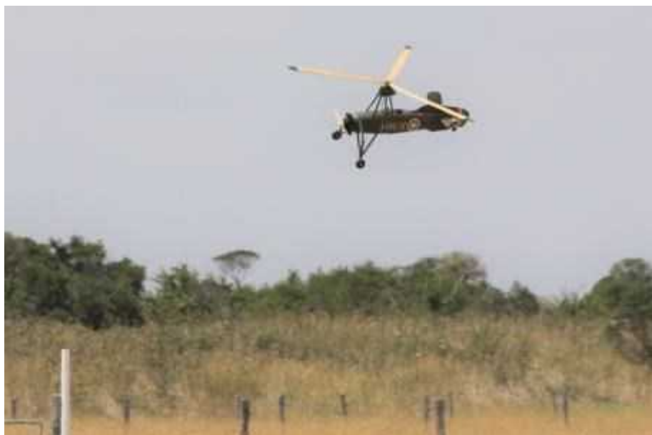
The nose down tight turn at low altitude that brought the model down.
