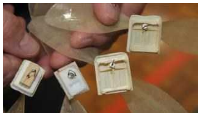
Otto's continual search for lightness even carried over to the noseblocks on his models.
