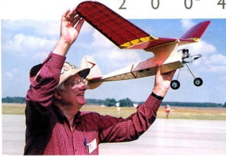
Tandy Walker (Arlington TX) scaled his Lanzo Bomber down to a 55-inch span to compete in Class A and B. Power is a Shilen OT .19 Ignition engine. Covering is Polyspan.
